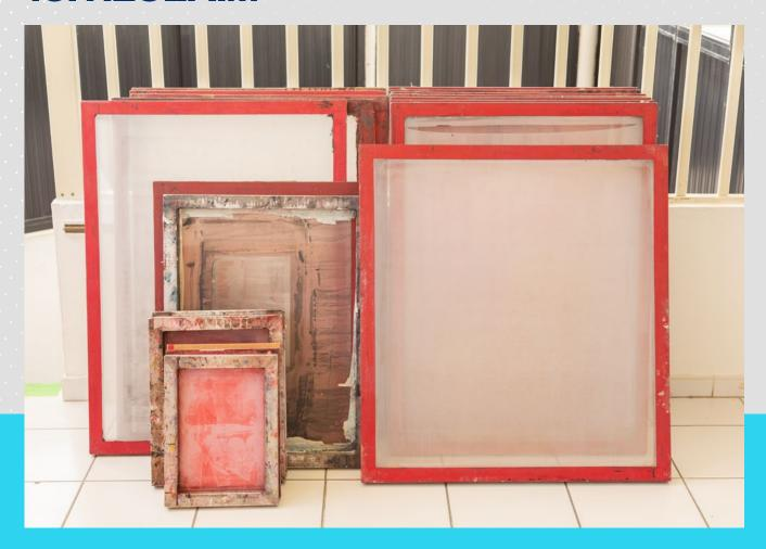
**Reclaiming** involves removing the old stencil and emulsion from a screen so it can be reused for a new design. This **process** typically uses chemicals to dissolve the emulsion, allowing the mesh to return to its original state. This can be done with Easiway's **Dip Tank** solution. Dip Tanks automate a lot of the grunt work that takes a lot more time reclaiming manually.
